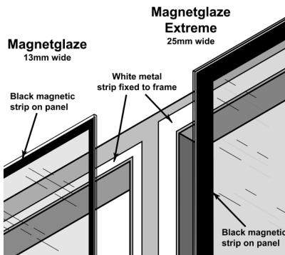
**HELPFUL HINTS** - For larger windows (1200mm x 1200mm or bigger) we strongly recommend placing a couple of screws under the glazing panel to support the sheet. This will remove the risk of the sheet from slipping down and becoming detached. Alternatively, consider using new Magnetglaze Extreme.
